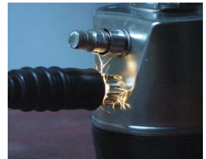
POWERCELL PDX load cell under laboratory testing of a simulated lightning strike.
