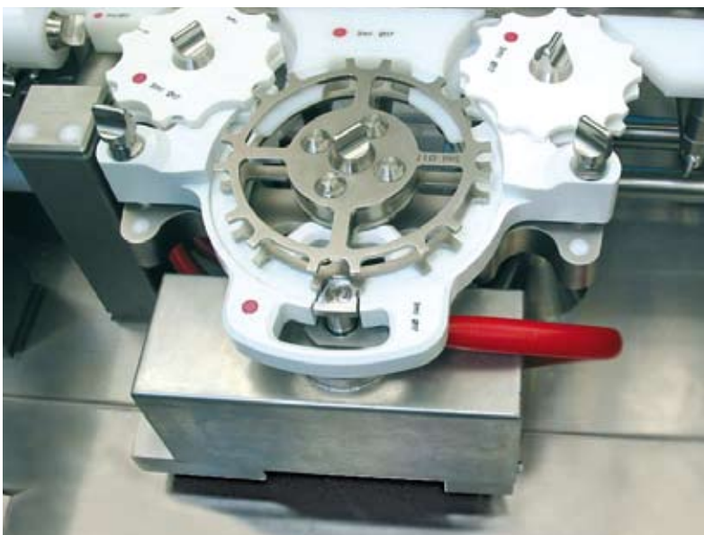
Weighing module integrated in a pharmaceutical filling machine. (Picture: Groninger & Co. GmbH, Germany)
