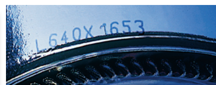
Lightjet Vector Scribing laser High quality mode (stroke fonts)
