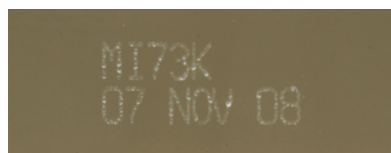
SmartLase 130i Dot matrix laser Rapid mode (7x5 dots)
