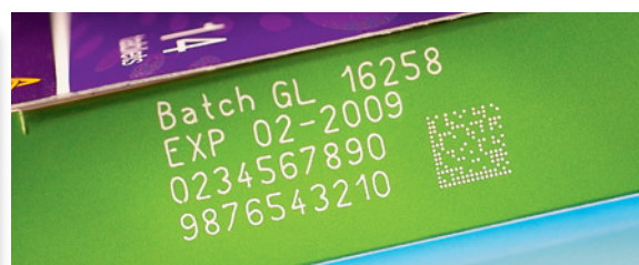
Lightjet Vector Scribing laser Serialization coding (stroke font, Datamatrix 16x16)
