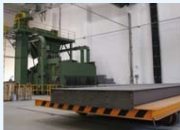
The steel in the VTS320 is shot blasted to create a fantastic painting surface
