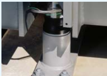
Optional risers elevate the scale for more bottom clearance and easier cleaning
