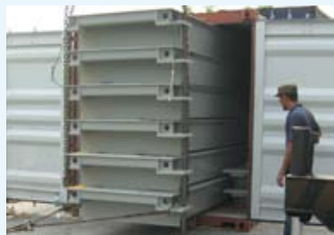
The VTS fits easily into a standard sea container or on a flat bed truck
