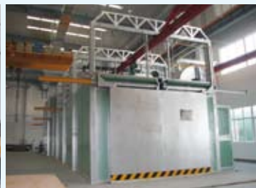
The VTS320 is epoxy painted and temperature cured eliminate corrosion
