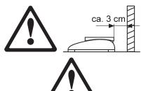
If the **power cord** is damaged, the scale must no longer be operated. Therefore check the cable regularly and ensure that a free space of about 3 cm is left at the rear of the scale, so that the cable is not kinked too severely.
