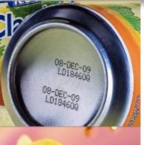
Printing on all types of substrates Print speed up to 8 m/s
