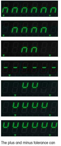
The plus and minus tolerance can be selected separately. The classifications are multiples of the selected tolerance.
